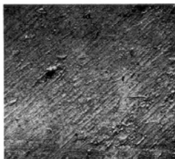
In addition to the ball bearing action, Monolec greatly increases the film strength of a lubricant through particulate attraction. To measure only the wear-reducing ability of the Monolec additive, a radioactive wear test was conducted. Visible proof of Monolec's ability to reduce wear is seen in the photomicrographs in Figures 3 and 4.
