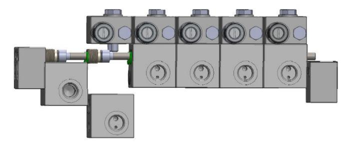
FINAL BASE INTERMEDIATE BASE FOR AIR INLET INTERMEDIATE BASE FOR AIR OIL OUTLET
