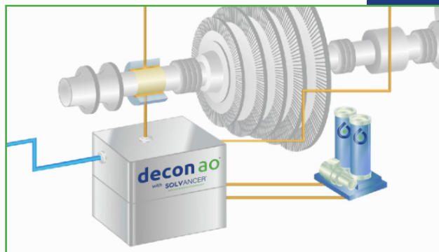
ESP removes the Varnish from the oil and DECON AO replenishes antioxidants
