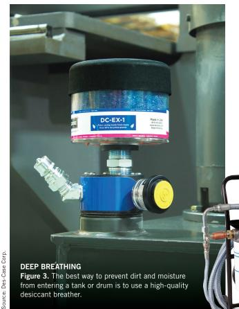
Systems like these allow staff to easily clean new oil, keep it clean, prevent cross-contamination, and track lubricant consumption by product type without having to engineer the process from scratch.
