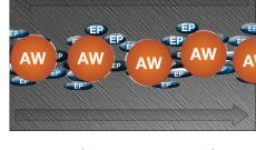
boundary conditions are present. As heat increases, Duolec is activated, working in stages to provide a dual layer of AW and EP protection. In EHD and mixed film conditions, the AW components of Duolec kick in. After loads become even greater, the EP performance is activated. When incorporated into gear oils, Duolec reacts quickly with the changing conditions to provide protection. The friction- and wear-reducing capabilities of Duolec can be seen in the test results on the next page.
