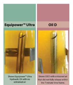
This test measures the time for entrained air content to fall to a relatively low value. Entrained air in hydraulic oil can cause sponginess and lack of sensitivity of the control of turbine and hydraulic systems. It is critical that hydraulic fluid has the ability to separate entrained air from oil.
